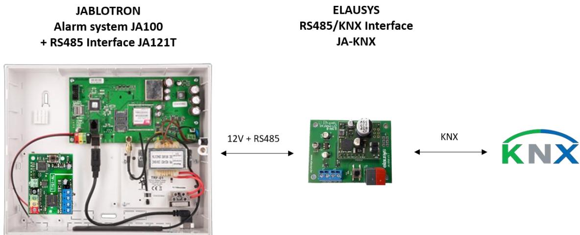
NOTE: When a user is logged in service mode on the alarm system, the RS485 and KNX interface are disabled.
